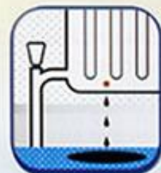
Pin holed radiators
