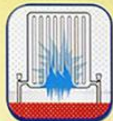
Radiators with cold panels
